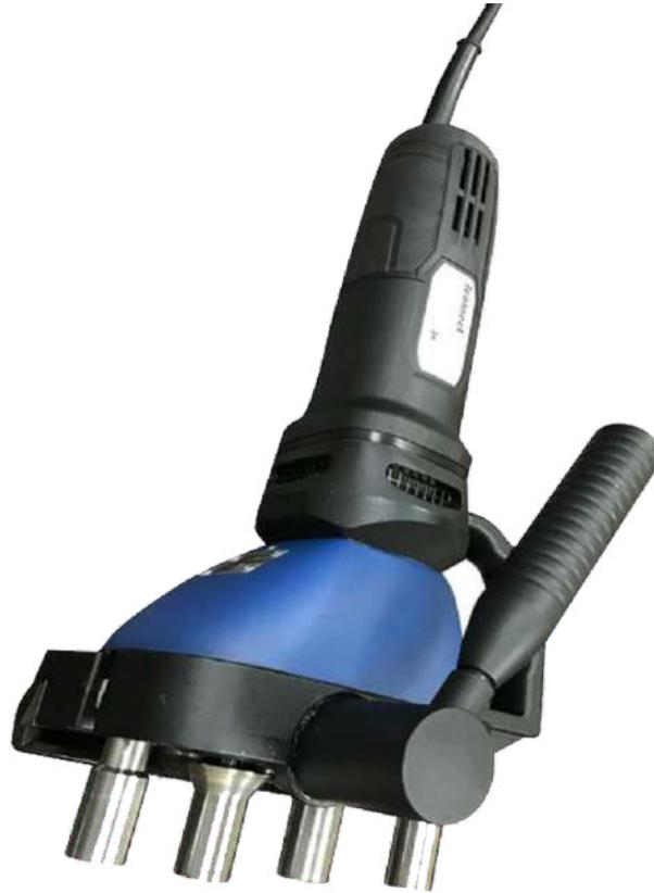
DUCTFAB, Pittsburgh Lock Closer - Electric Operated. There are two models-SC 10 with max capacity 1mm and SC 12 with max capacity 1.2mm. They are the ideal machines for use with Lockformers/Rollformers for closing straight or curved Pittsburgh Lock seams on ducting. Automatically adjusts to the thickness of metal sheet. The Seam Closers/Lockers are powered by a 1400 watt speed adjustable motor, enabling the user to achieve high quality and tightly joined seams with ease
