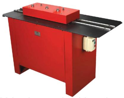
Used for joining sheet metal at right angles on straight runs. This is a more sophisticated joint than the Pittsburgh lock, requiring less labour. The male section snaps tightly into the female with an almost unbreakable joint.
