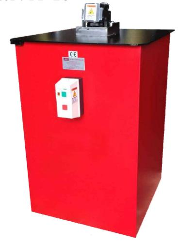
DUCTFAB 16swg (1.6mm) POWER FLANGERS are principally used for forming a right angle flange on curved, straightand irregular shapes. These machines are fitted with a tilting head to enable complete circles to be formed. DUCTFAB Power Flangers are manufactured with hardened top plates, shafts, forming rolls, gears and guide fences.
